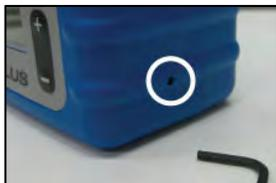
**Note:** Flow range select must be in Lo if the flow is less than 450 cc/min and in Hi for rates from 450 to 5000 cc/min. The flow range select is on the right side of the case and can be switched between Lo and Hi with a 2mm (5/64") hex wrench supplied with the pump. Indication of Lo or Hi selection displays in the middle of the lower display status line.
