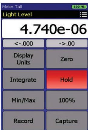
**Meter Screen** provides a large numerical display which allows customers to easily view the measurement data. While using Meter, customers can also perform many processes including:
