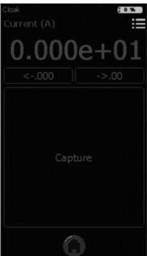
**Cloak** limits the amount of light added to the environment during test. It was designed to allow taking measurements in a dark environment as easy as possible without compromising the results. Simply touch the oversized sample button and a single reading will be stored into the internal memory.
