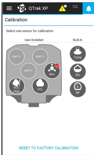
An Out-of-Range error during the calibration of a sensor means the sensor's offset or calibration slope adjustment has drifted outside of the TSI<sup>®</sup> recommended specification for continued use. Sensor should be replaced or sent to TSI<sup>®</sup> for re-calibration.
