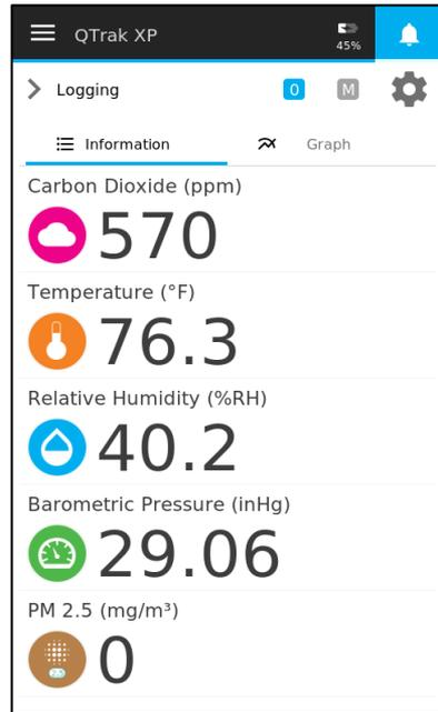
Selecting **Graph** presents real-time readings in a graphical format while selecting **Information** present data in a numerical format. To view sensors not shown on the page, swipe up and down.
