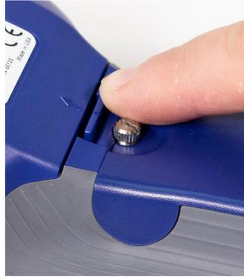
3. Turn the instrument over and hold it as shown while continuing to press on the release tab as previously described.
