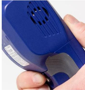
4. Press downward with both thumbs while holding the release tab above the back-cover. This requires some steady force.
