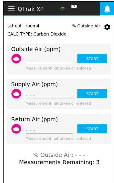
Three measurements are necessary for % Outside Air calculations - **Outside Air**, **Supply Air**, and **Return Air**. The measurements may be taken in any order. The calculation is performed once the final measurement is taken.
