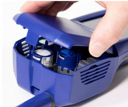
**Step 2 – Place the calibration cap onto the gas sensor you want to calibrate**
