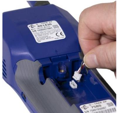
3. Insert the battery as shown in the picture, keeping the battery wires to the side and clear of the battery cover screw.
