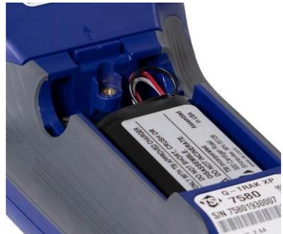
4. Attach the battery compartment cover, ensuring battery wires are clear of the screw.
