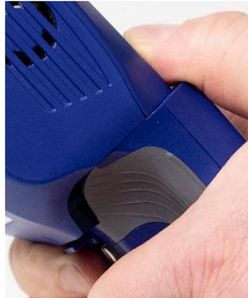
5. Continue to press down until the sensor module is free from the handle.
