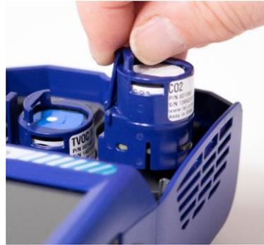
3. Position the sensor as shown, making certain the pins make good contact with the device. Gas sensors can be installed in any available slot. Listen for a click to confirm sensor is connected properly.
