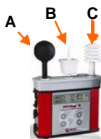
A. Globe thermometer B. Natural wet bulb thermometer C. Dry bulb thermometer
