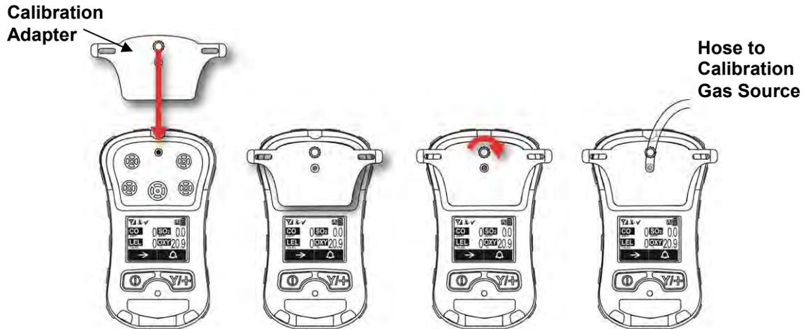
1. Align the Calibration Adapter's main body with the indented area around the QRAE 3's gas inlets.
