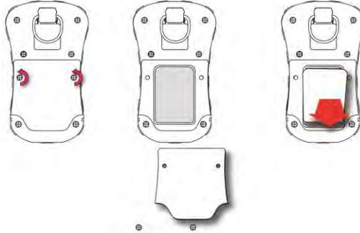
2. Remove the cover plate by tilting up the end closest to the belt clip and lifting off.
