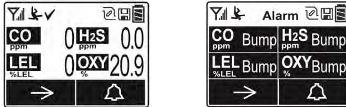
A bump test is required if the defined period of time between bump tests has been exceeded. This interval is set by an administrator using ProRAE Studio II.
