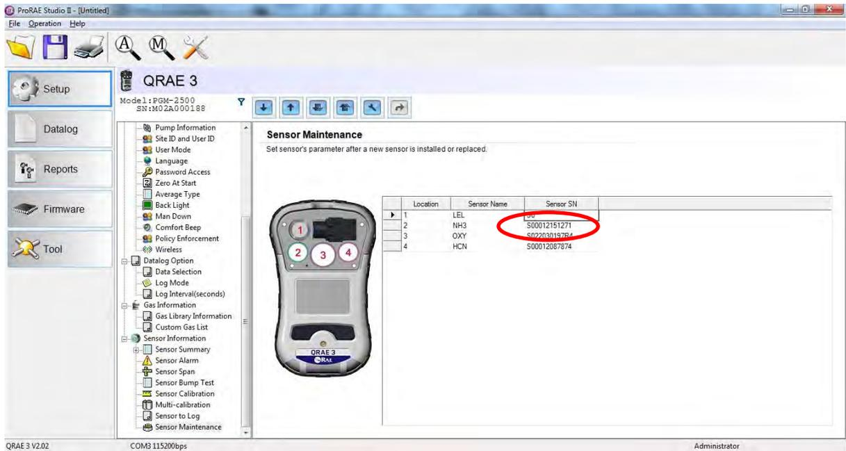
If you do not input all 10 digits of the sensor S/N, you will be alerted by red highlighting on the serial number text.
