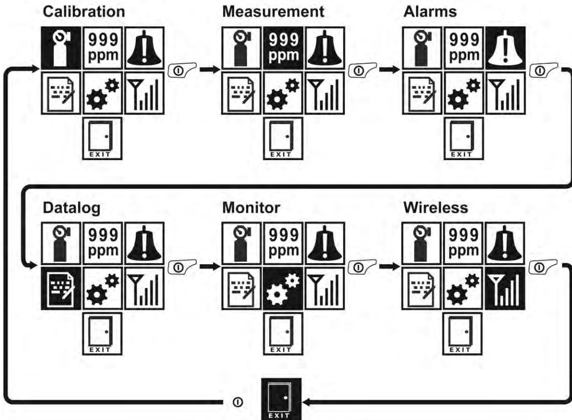
To enter a menu and view or edit parameters in its submenus, press [Y/+].
