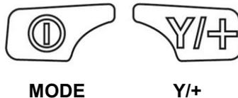
In addition to their labeled functions, the keys labeled [MODE] and [Y/+] act as “soft keys” that control different parameters and make different selections within the instrument’s menus. From menu to menu, each key controls a different parameter or makes a different selection.
