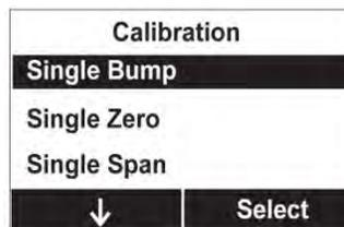
Each bump test or calibration option shows a countdown followed by sensor reading and pass/fail results.
