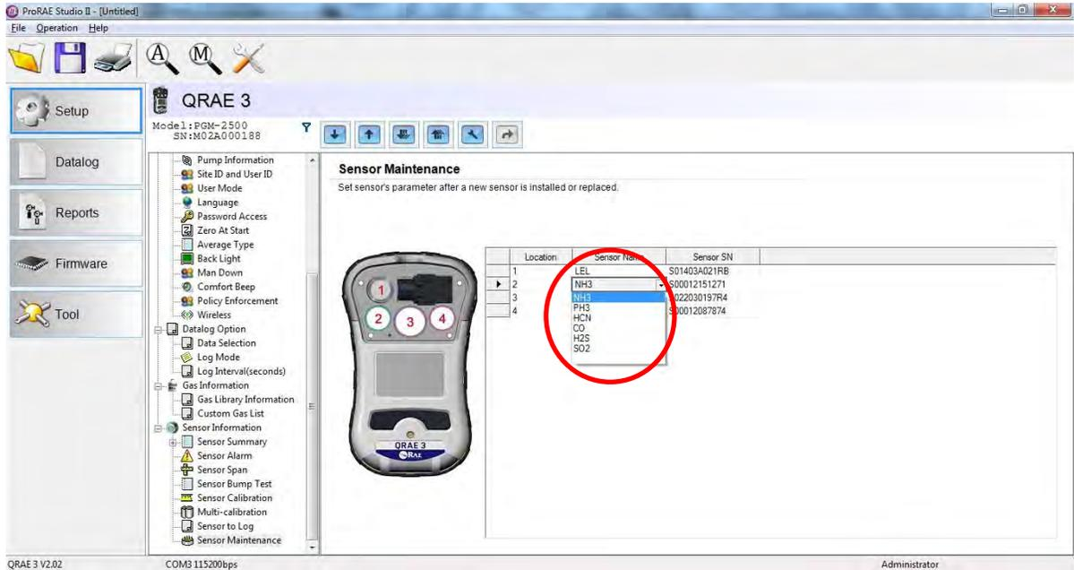
**Note:** For an updated PGM-2560/D, Slot 2 only supports Group N sensors, and not Group P sensors. Also, Slot 4 only supports Group P sensors.
