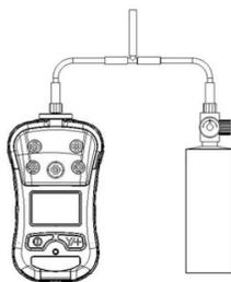
**Note: Make sure pressure in the calibration gas cylinder is higher than 100 psi when using a T calibration tube.**
