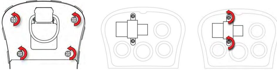
5. Press a new pump into place (a small amount of wiggling helps), making sure that both the inlet and outlet from the pump fit snugly over the two pipes.
