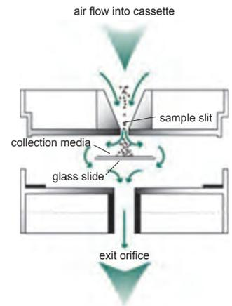
After sampling is completed, the cassettes are sent to a laboratory, where the slides are removed and direct microscopic analysis can be immediately performed. The collection media is compatible with a wide range of biological stains and refractive index oils, allowing direct qualitative and quantitative analysis of organic and inorganic particulate.
